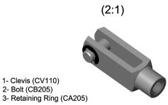
No sharp ends, no burrs, no significant surface defects. General Tolerances DIN ISO 2768-medium
